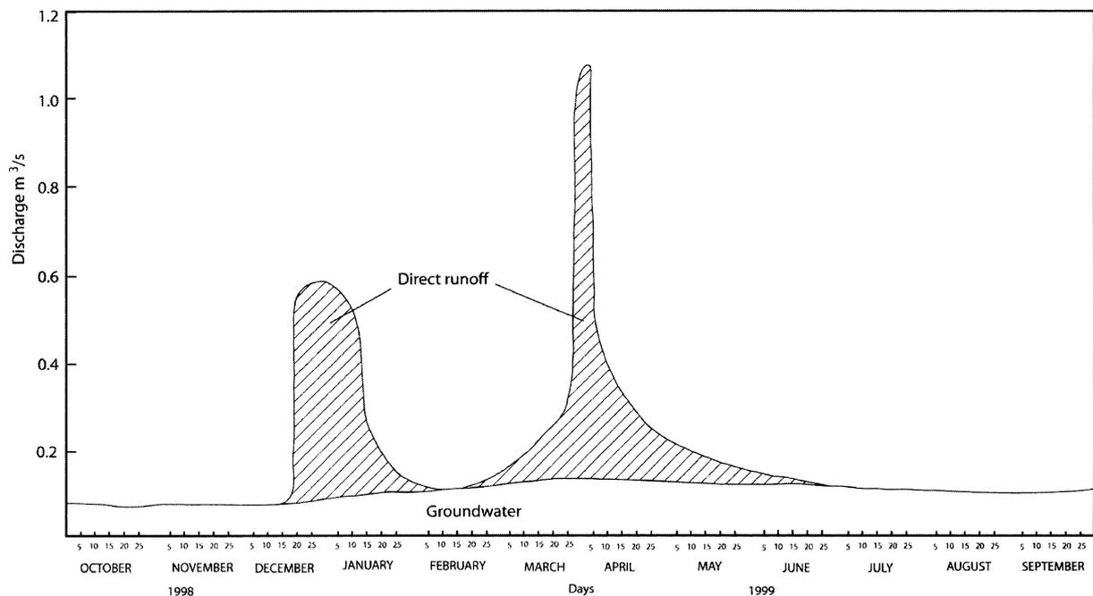
Figure 5. Stream flow hydrograph for Mwangongo watershed.
