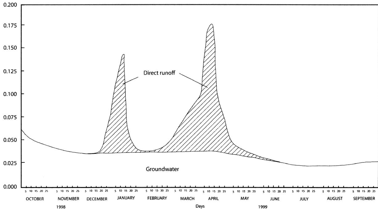
Figure 4. Stream flow hydrograph for Mitumba watershed.
