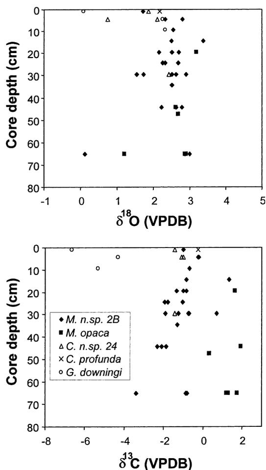
Figure 6. Oxygen and carbon isotope ratios for ostracode shells from core 86-DG-14 (Wells et al. 1999). Each measurement is of a single valve. Species names are listed in caption to Figure 8.
