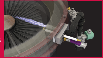
Patented Turbo Pilot 8,000 BTU/h Surefire Ignition System
