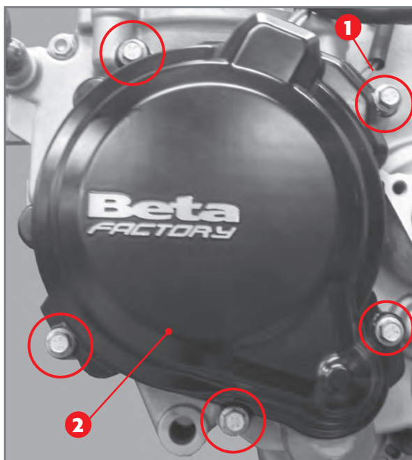
Fixing screws 1 of flywheel cover 2 .
