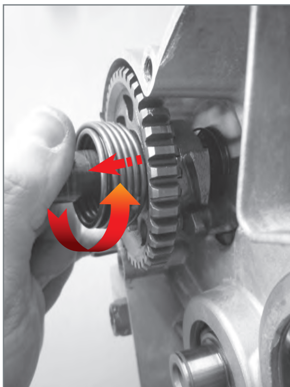
Extraction of shaft from crankcase.
