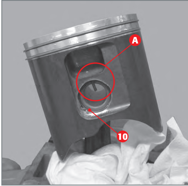
Removal of piston circlip.
