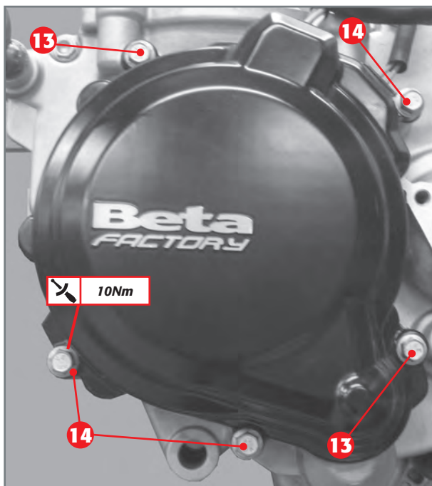
Flywheel cover coupled to crankcase.
