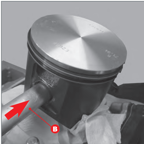
Removal of pin bolt.
