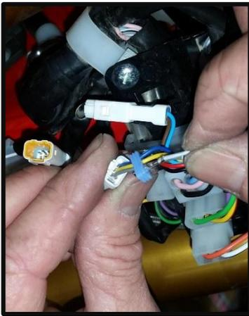
Pull the wire out of the rubber boot and push the rubber boot back into the connector. This will turn off the oil injection failure light on your dash.
