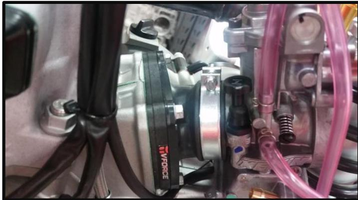
Remove the stock intake manifold and replace it with the new one supplied using the new gaskets. Re-install the slide into the carburetor and install the carburetor on the manifold. Install the subframe, rear air boot, and exhaust muffler.
