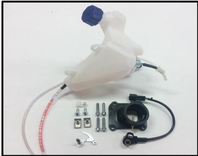
These are the parts that you have removed. Keep these parts all together in case you wish to reinstall the oil injection.
