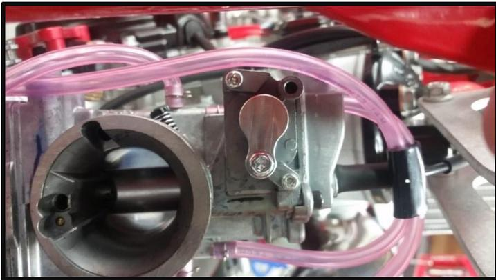
Reinstall the TPS plate (now without the lever) and the TPS plug that is included with this kit making sure the oring is in place.
