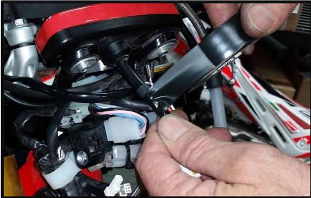
Using black electrical tape, tape up the wire to the wire loom to avoid it from contacting metal. This wire could just be cut however by taping it up, it can easily be reinstalled if needed.
