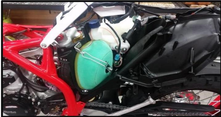
Start by removing the muffler, airbox bolts (the ones attached to the plastic part of the subframe) and the four rear subframe bolts holding the plastic part to the two aluminum uprights. Swing the plastic part of the sub frame up leaving the airbox in place. Remove the oil tank assembly including the oil pump and the low oil sensor (attached) along with the oil line going to the intake manifold
