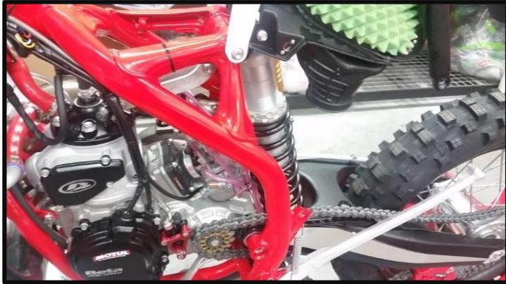
Re-install the top subframe to the uprights. Use blue locking agent to the four bolts that connect the plastic to the aluminum uprights. (do not use locking agent on the air box bolts) Next, remove the rear airboot clamp to the carburetor and the lower subframe bolts and swing the entire subframe and airbox upwards.
