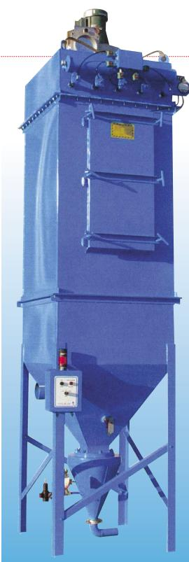
C&C Reclaim Systems efficiently recycle airborne product dust when silos are filled. Units operate automatically from a safe ground-level location – using dense phase conveying to minimize material degradation and component wear as they return product dust to silos.
