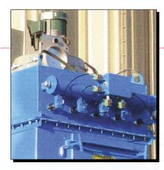
Exhaust Fan draws particle-laden silo air through the dust collector.
