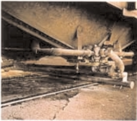
FOR AIRSLIDE CARS INCLUDING AIR MANIFOLD FOR THE CAR.
