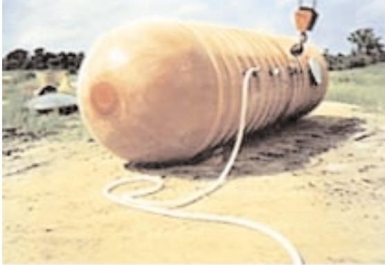
*Tank being tested with 11 1/2" of vacuum prior to delivery.*
