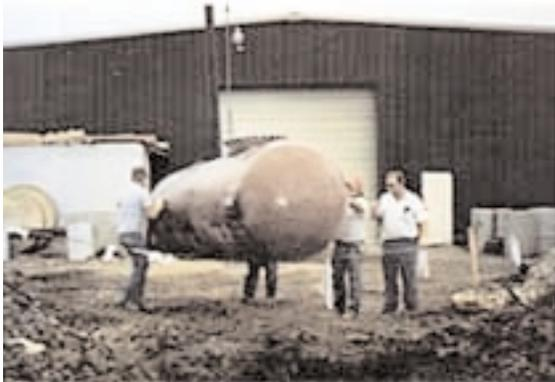
*Preparing 1,000 gallon double wall tank for UL test.*
