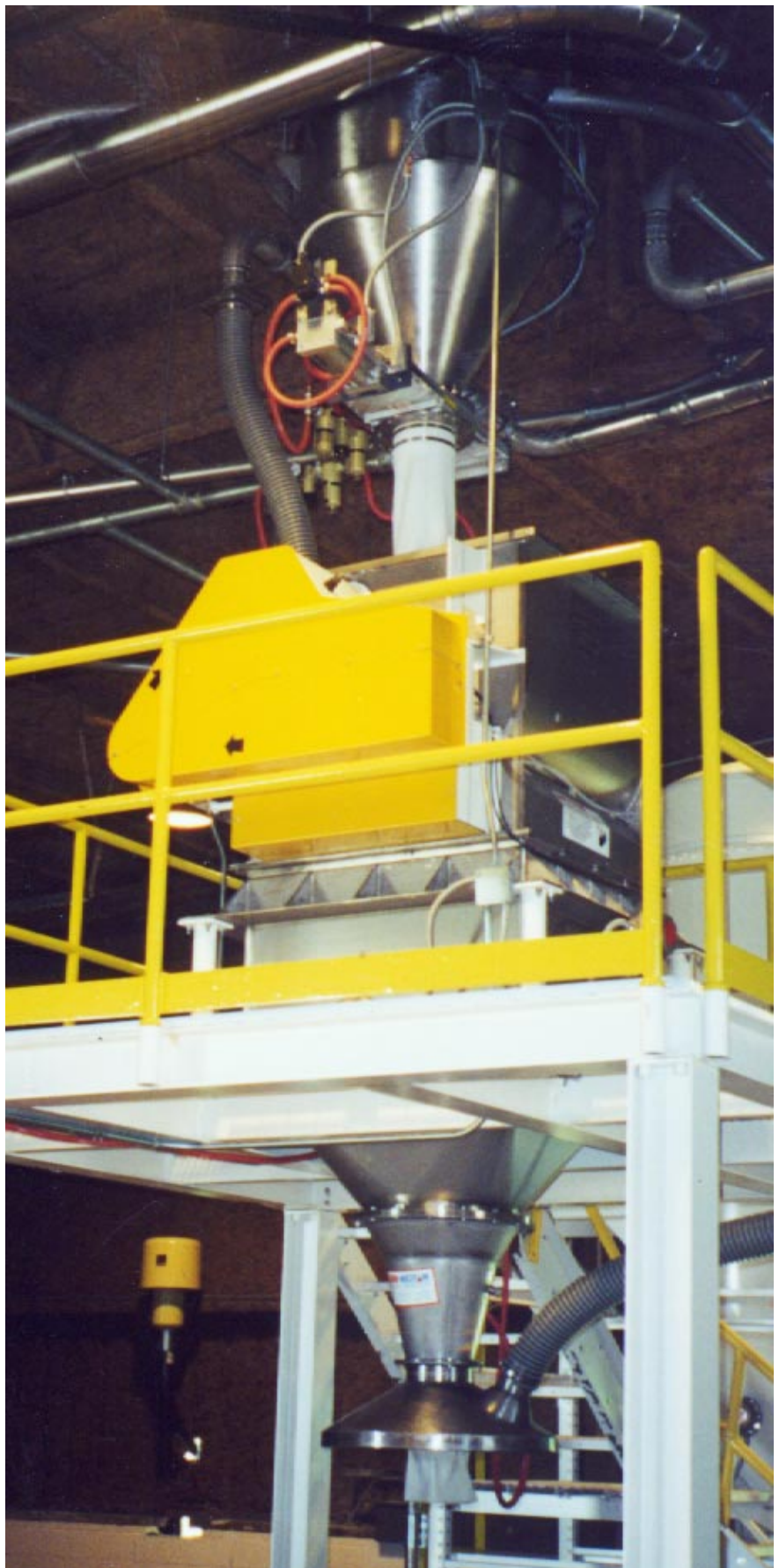
Typical system consisting of scale hopper, Forberg fluidized zone mixer, transition hopper to dust control hood for filling IBC's.
