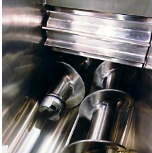
Timed Augers And Auger Feed Roller For Block Or Bulk Products
