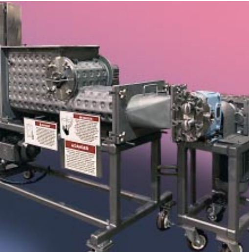
Dual Chamber ASME High Pressure Dimpled Jacket
