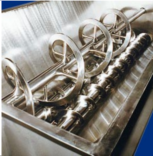
Agitated Leveling Ribbon To Reduce Bridging Or Product Segregation
