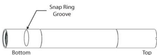
**C.** Insert Snap Ring (14) into bottom of Cylinder (12). Ensure that it sits in the snap ring groove.
