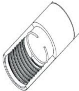
**D.** Insert Bottom Spacer (15) into bottom of Cylinder (12). Ensure it sits up against Snap Ring (14).
