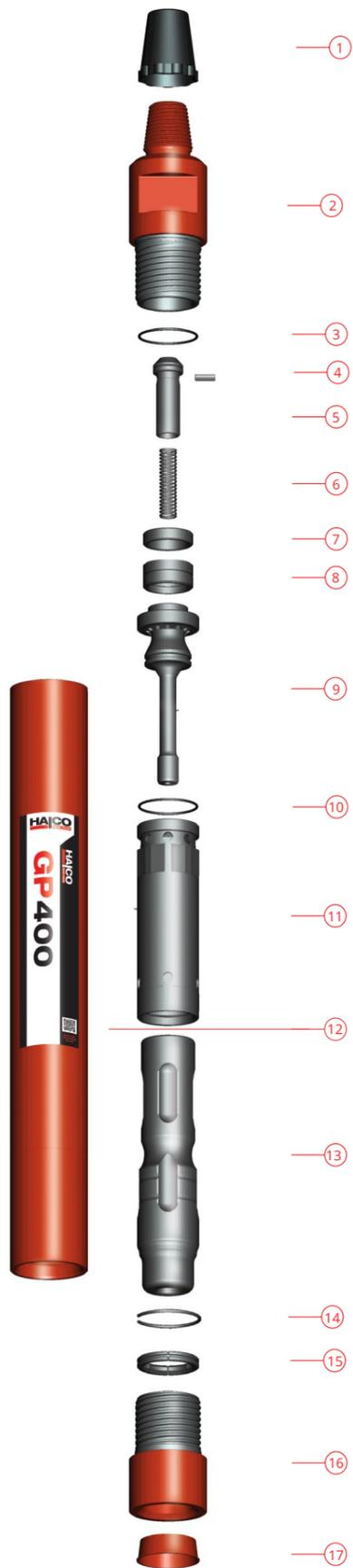
**C.** Insert Liner (11) into top of Cylinder (12). Ensure it sits against the shoulder of the Cylinder (12).
