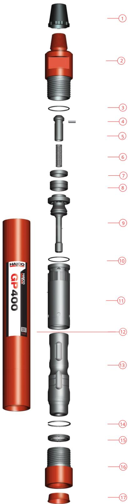
**B.** Break the top joint between the Cylinder (12) and Top Adaptor (2) and bottom joint between Cylinder (12) and Chuck (16).
