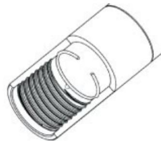
**K.** Grease splines and fit Chuck (16) over the Drill Bit.
