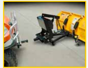
Step 4: Roll the plow away
