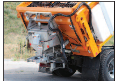
Salt Slurry Generator
