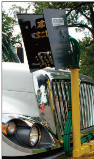
Spray Head: Front, Mid or Rear Mounted. Multi-Zone Spray Load with 30° Linear Actuation Tilt to Follow Ground Contour.
