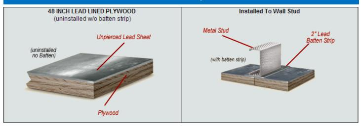
**Lead Lined Plywood** is constructed of a single roll of our own lead sheet, meeting federal specification QQ-L-201 F or ASTM B 749-03 for lead that is laminated to ½", 5/8", ¾" or 1" Fire Resistant plywood. The thickness of the plywood is determined by the lead thickness requirements for the level of radiation shielding your construction calls for. Leaded plywood is an excellent way to construct radiation shielded rooms.
