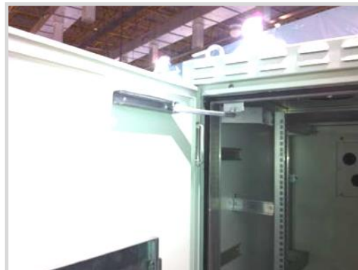
Fig 2: inside of the cabinet shielded with gasket EMI RFI and IP.
