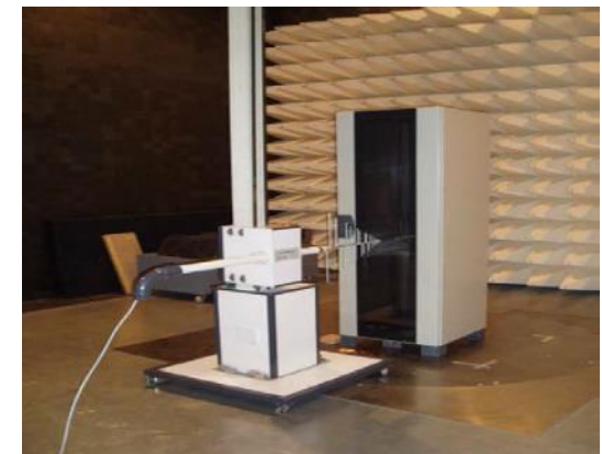
Fig 3: Testing of a cabinet in a shielded room
