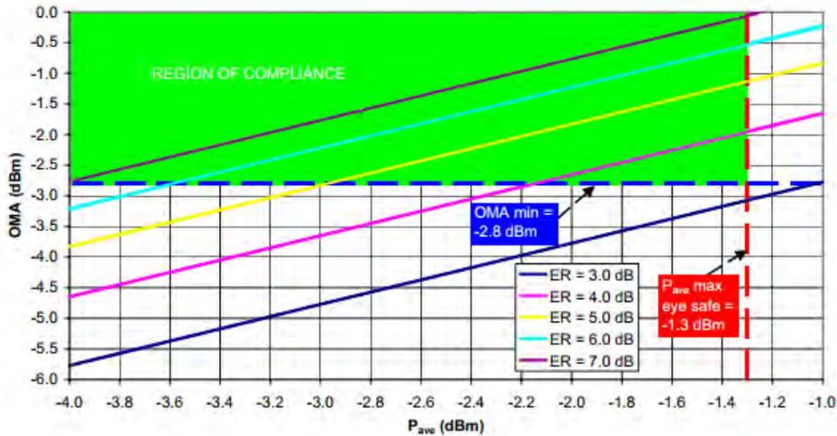
Then, for every transmission link configuration a region of compliance can be defined, setting the range of values that Er, OMA and Pavg need to comply with to fulfill the targeted standard.
