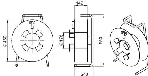
Gantry drum, with braking device and handle crank
