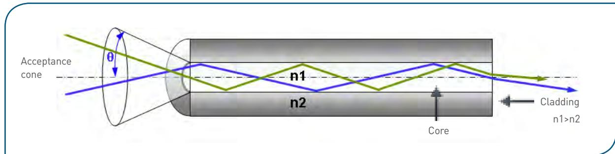
The light rays are totally reflected by the cylindrical surface between the core and the cladding because of their different refractive index. To confine the light (the optical signal) into the core, the refractive index of the cladding must be lower than that of the core:  $n_1 > n_2$ .
