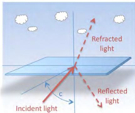
Light is partially reflected and partially refracted because its angle of incidence is inferior to the critical angle.
