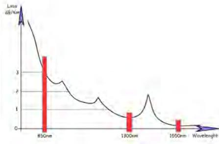
For Telecommunication and for glass optical fibers, we use light in the infrared region, typically around 850, 1300 and 1550 nm due to low attenuation of the glass fiber at those wavelengths.
