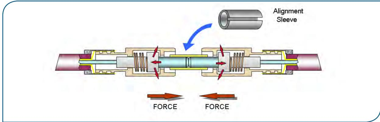
The ferrules of the plugs are aligned into a guiding sleeve belonging to the adapter.
