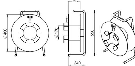
Gantry drum, with braking device and handle crank
