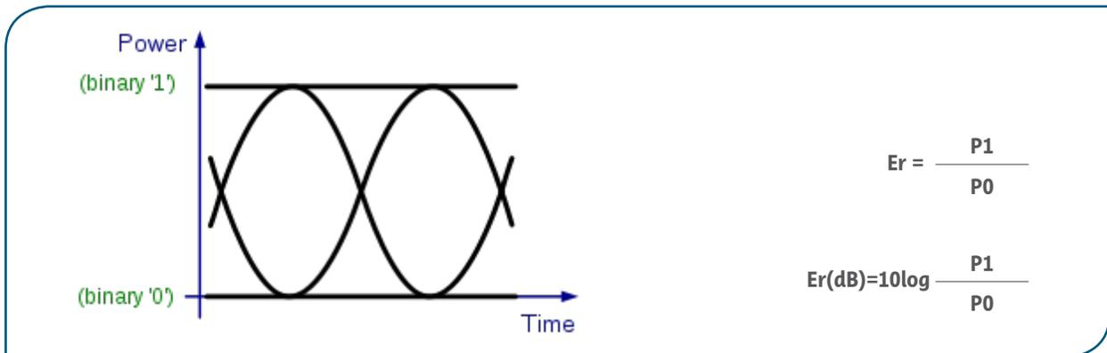
In an ideal transmitter  $P_0$  would be zero, but in most practical its lower value is limited by the laser threshold. For data link optimization, ER is set by manufacturers at the best compromise between the transmitter optical power requirement and the bit error rate of the link. The Optical Modulation Amplitude, OMA, is defined as the difference between the high and low levels :
