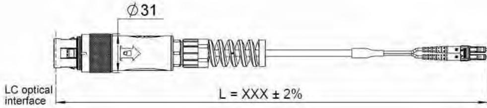
Any configuration of pre-mounted optical cable assembly with OSIS® is available on upon request:
