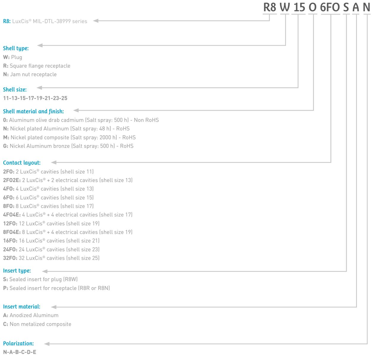
All connectors are supplied with a plastic cap. All connectors are delivered without contacts.
