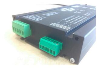
NOTE: In the photo, the input voltage connector and the input current sensors one are shown.
