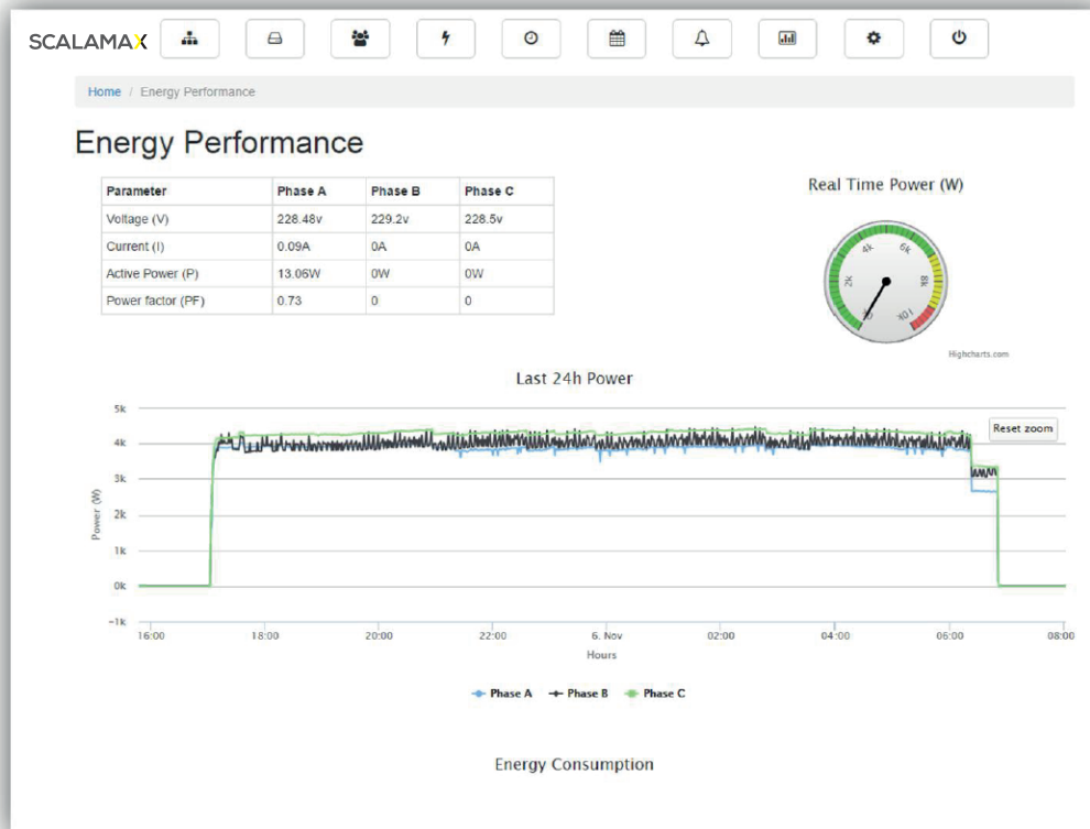
Figure 2: Screen showing power consumption for the past 24h
