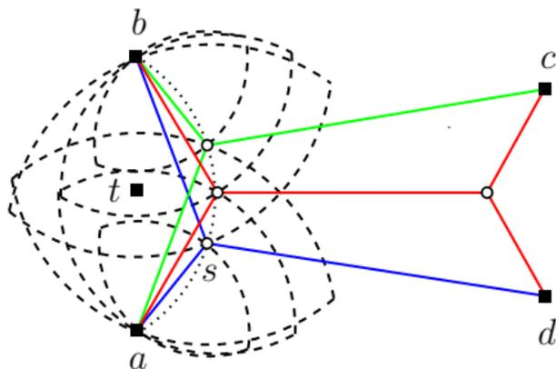
For example, suppose there is a fifth terminal  $t$  halfway between  $a$  and  $b$ . No matter where  $s$  is located on  $\widehat{ab}$ , terminal  $t$  would be inside one of the two lunes defined by edges  $as$  and  $bs$ . Hence, none of the three FSTs shown in the figure would be generated.
