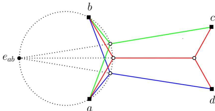
Consider the three FSTs in the figure. The terminal pair  $\{a, b\}$  forms a cherry in each of these FSTs, and the Steiner points are located on a common Steiner arc  $\widehat{ab}$ . Here the three FSTs share a sub-topology (the cherry  $\{a, b\}$ ) and the same equilateral point  $e_{ab}$ .
