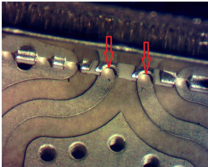
Note: a hot plate and/or hot air re-work station could also be used instead of (or in conjunction with) the tweezer/exacto-blade method outlined above. Realize that the splitters were constructed with low temperature/lead-free solder so that a hot plate high temperature should not exceed 160 C.
