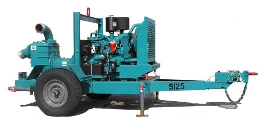
All trash pumps have the ability to be used in conditions with intermittent flows and suction lifts up to 25 feet. This is possible due to CDPW's unique oil bath system which provides constant lubrication to the bearings and mechanical seal.
