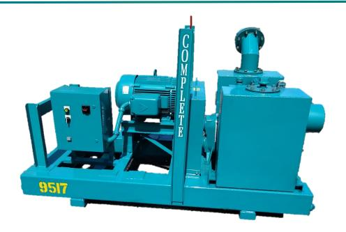
protect pump end components during periods of dry run and reduce surges in discharge and header lines. And since the rotary lobe pump end handles both the air and water together, there is less maintenance required than with priming assisted pumps. A motor mounted gear drive reliably transfers power to the industry leading all cast iron Vogelsang wet-end. Optional Piggy-Back V-belt drive system available.
