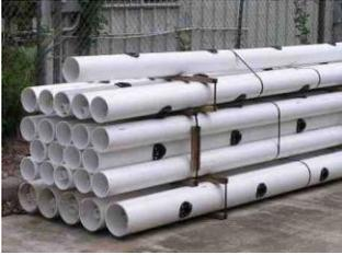
Sch. 40 pvc header pipe with our standard configuration of 7 header saddles per 20' section of pipe (approx. 3' spacing of saddles).
