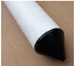
2" x 20' PR160 pvc wellpoint, bottom 3' is slotted .015" and has an inner draw down tube for maximum draw down efficiency. Wellpoints can be ordered any length to 23'.
