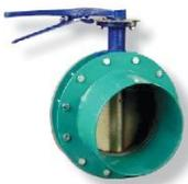
Butterfly valves are made of PVC with multi-position adjusting handle. The valves are used to isolate sections of system and seal off the suction from backup pumps when replacing pumps. Sleeveable flanges make it easy to connect to the pumps and header, just like the fittings.
