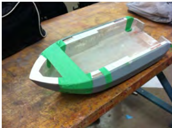
-After sanding reserve buoyancy parts, they were epoxyed under tension and let to cure over night
