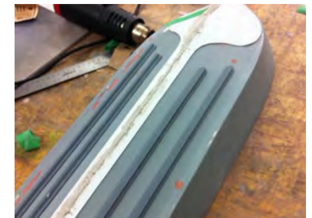
-Cut T plastics extrusions and glued to hull
