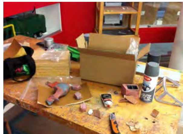
-Spot putty and filler primer the 3D printed parts
