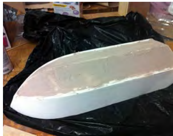
-Bondo surface of hull
