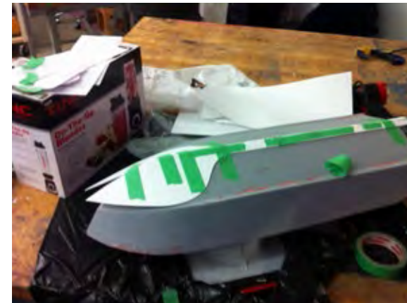
-Cut 1/16" thick plastic into two profiles
