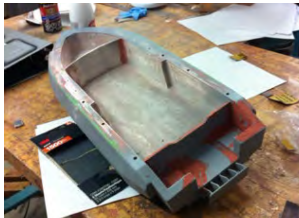
-Interior walls / bow cut out of plastic and mounted into the interior
