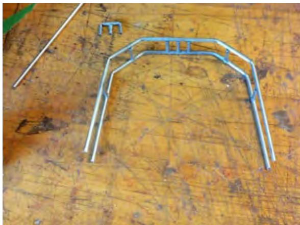
-Bent 1/8" diameter aluminum tubing for several of the details
