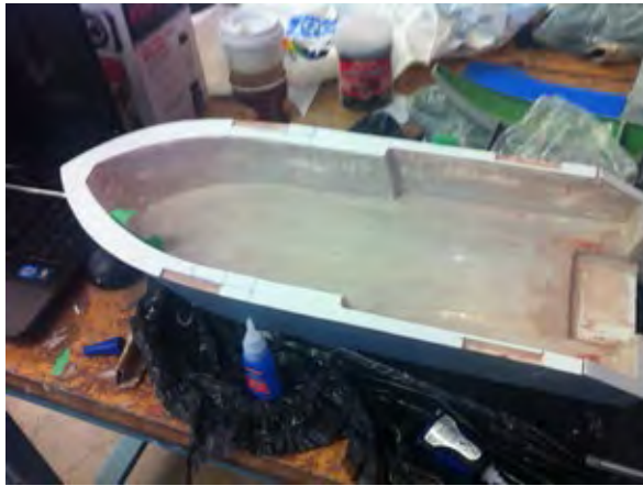
-Cut 1/16" thick plastic for the gunnel
