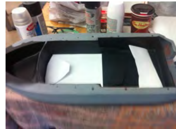
-Interior was sprayed with a matte finish paint. -Paper templates were cut out in order to skin the floor
