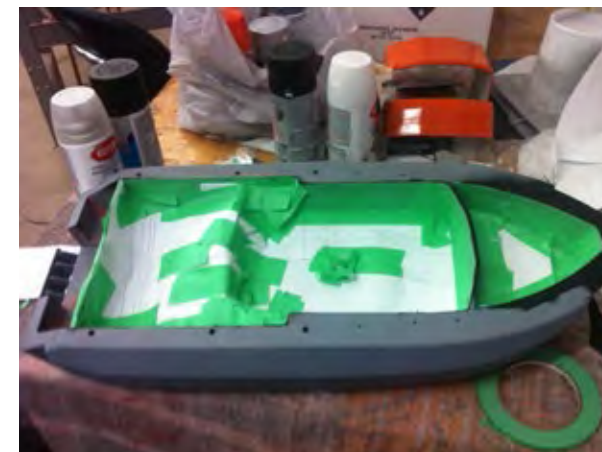
-Interior was masked off to then paint the exterior
