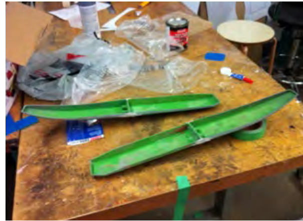
-Glued the reserve buoyancy parts together
