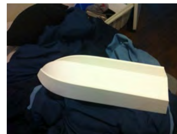
-Hull CNC out of EPS foam
