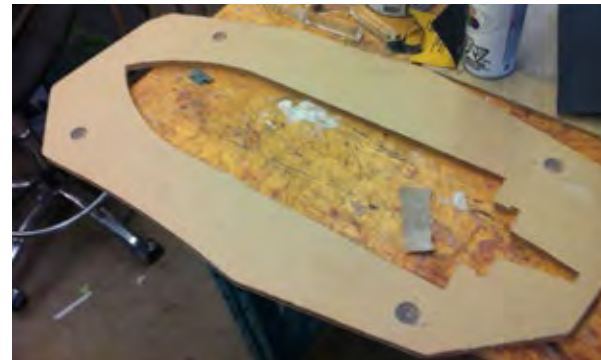
-CNC .50" thick acrylic for base -Drill holes for .50" diameter clear acrylic dowel
