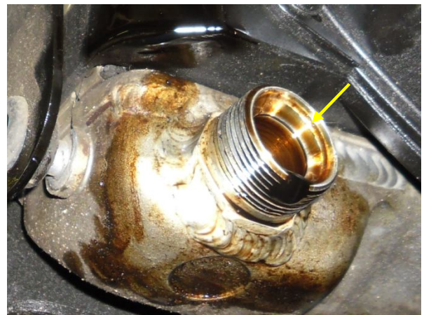
This sealing surface is damaged.
