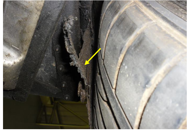
The front wheel inner cover has been worn away.
