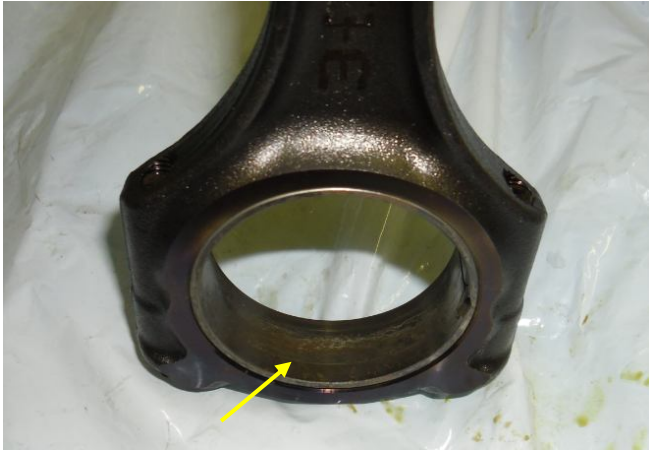
Big end bearings have lubrication failure damage
