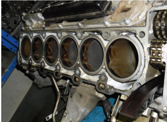
The right bank of cylinders has experienced four point thermal seizures in all six cylinders
