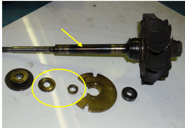
The turbine shaft and bearings of the left bank turbo charger.
