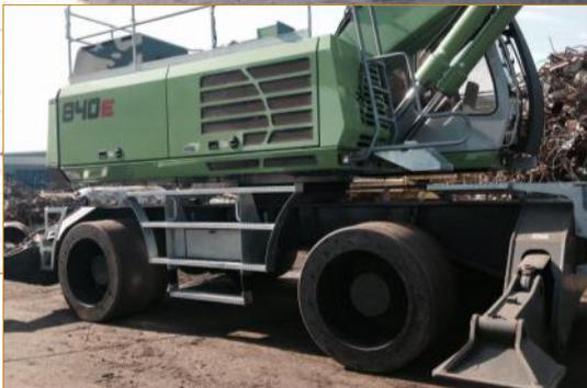
SETCO’s “Super Single” material handler tyre assemblies come in many different sizes and can replace any dual wheel assembly! Available as slicks or with traction tread, SETCO can build a tyre customized to your needs!
