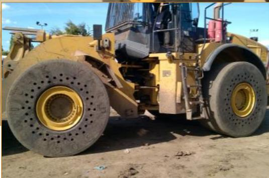
Using the same quality 100% natural rubber compounds found in SETCO's expanded-rim solid tyres, you can expect a premium product at a much lower cost while using an OEM rim. SETCO offers a rim exchange program, delivering the tyres pressed on to rims to you for quick mounting with minimal downtime.
