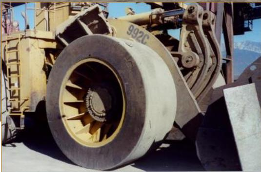
SETCO's expanded rim solid tyres are designed for the toughest environments where traditional press-on tyres would fail. Using 100% natural rubber for its superior wear and cut resistance, SETCO's expanded-rim solid tyres will withstand even the toughest load and carry scrap and waste operations.
