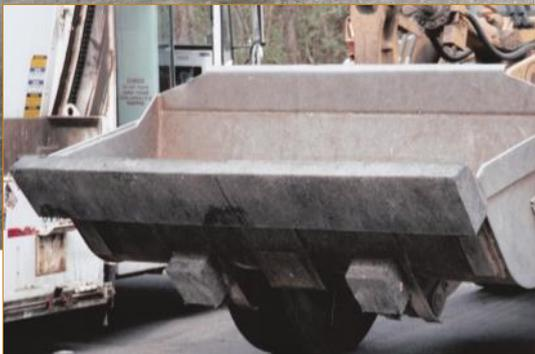
SETCO's rubber cutting edges are made from durable natural rubber that unlike steel, will not wear out your concrete and will not spark. The rubber also acts as a sponge that keeps the floor drier, thereby increasing the traction of solid tyres. Tapered on both sides, the rubber cutting edges are even reversible!
