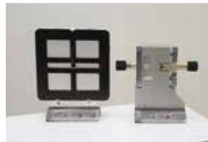
Sample fixtures with dovetail guide
