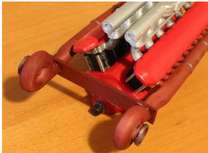
There are 4 tubes with 90 degree bends. These are used to connect the turbo cold ends to the intake tubes. There is a longer tube, a medium long tube and two shorter tubes. (The short tubes may be changed to be the same size).
