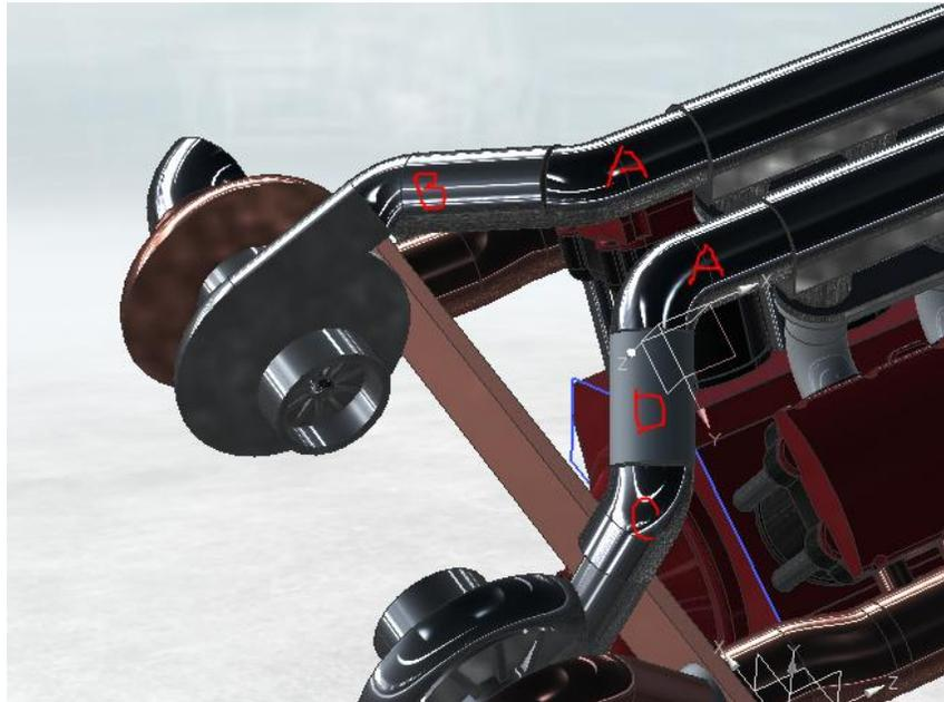
The short 45 degree angle tube "C" mounts on the right side turbo. The straight tube mounts is marked as D on the image to the right and bridges between the short tube and the tube "A" on the right side (from the back) turbo.
