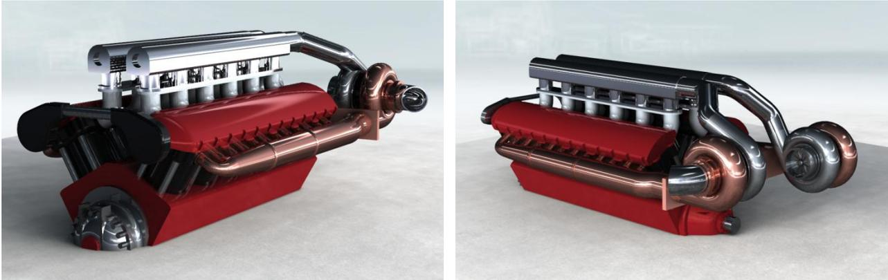
There are two different turbo hot end pieces - one with a slight bend and one that is straight. They glue to the cross beam and match up with the exhaust tubes. The angled side goes on the right hand side of the motor looking from the back as in the picture to the right.
