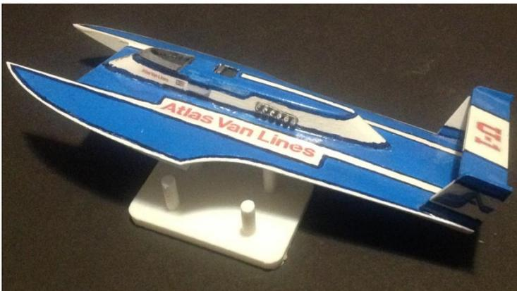
Attach the intake scoops behind the cockpit. The longer edge of the scoop is the top side of the intake.
