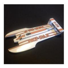
Attach the upper and lower sections of the hull using CA glue and aligning the pieces to be even at the transom
