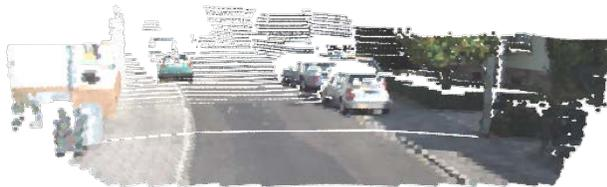
Fig. 6. A velodyne scan coloured by one of the KITTI cameras.
