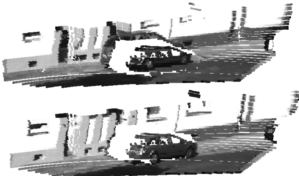
Figure 5.7 – These images show a camera image from the KITTI dataset projected onto its corresponding Velodyne scan. The top image shows the result obtained by the motion only approach, while accurate rotation values have been estimated there is significant uncertainty and error in the translation. The bottom image shows the combined approach where the motion method has constrained an appearance-based optimisation, allowing a superior calibration to be obtained.
