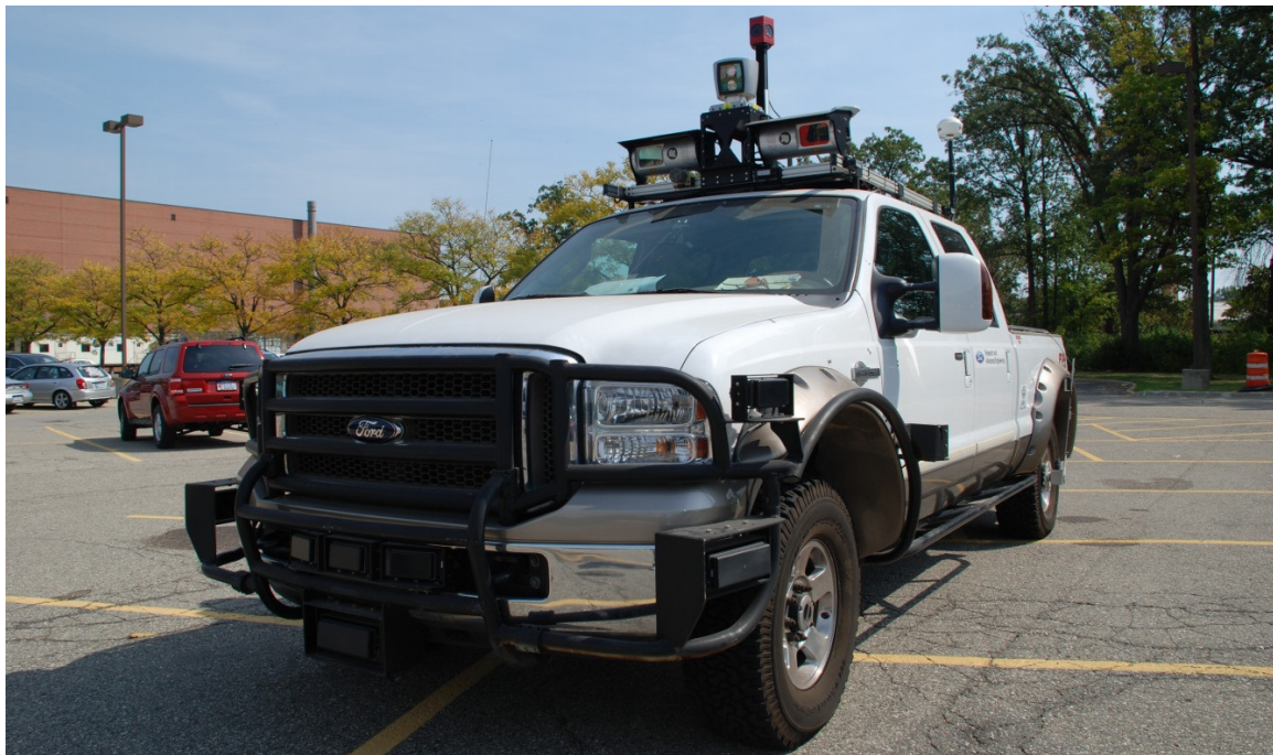
Figure 6.2 – The system used to gather the Ford campus vision and lidar dataset.
