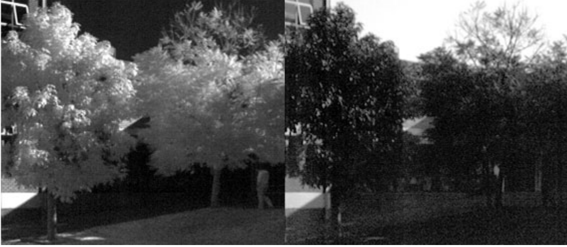
Figure 3.7 – A pair of example images showing how gradients may reverse direction between modalities. In the left image, taken at 950 nm, the trees are white with a black sky behind them. However in the right image, taken at 418 nm, the trees appear black and the sky white. This means that if the gradient between the trees and sky is calculated, the gradients will be 180 degrees out of phase for the two images.
