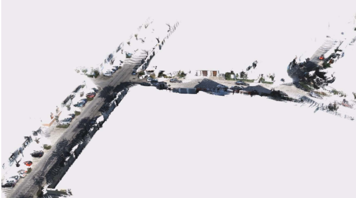
Figure C.1 – A section of a coloured 3D point cloud generated using the lidar, cameras and GPS/INS systems of the KITTI system.
