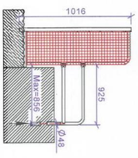
Insert the Leg of "F" Frame into the Deck Hole Anchors which you casted in the concrete (pls as close to pool edge as possible) two weeks ago to install the Wall Goal to the Pool.
