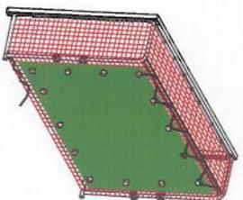
Use the White Rope to traverse the holes of Canvass to fix the Canvass to the Bottom Frame, Side Frame and Top Tube, then fix the Red Net to the Eyebits and lace it around the Side "L" Frames with White Rope.
