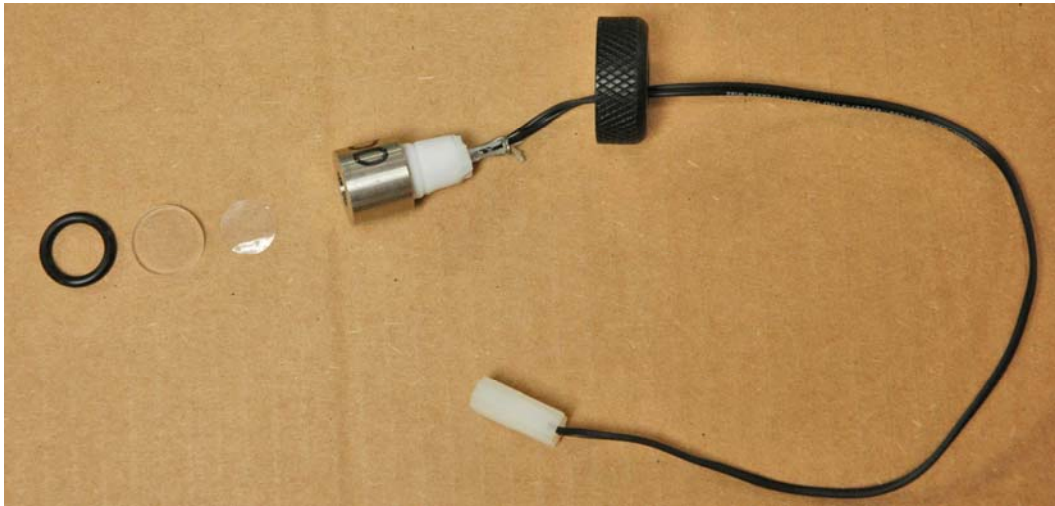
Figure 3.2 UV Sensor Assembly for PVC Units
