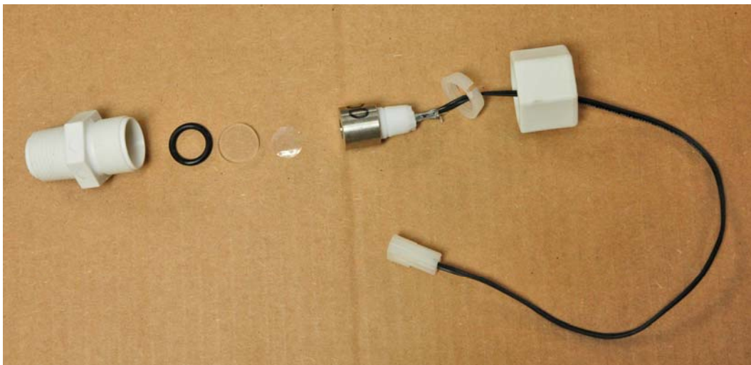
Figure 3.2 UV Sensor Assembly for PVC Units
