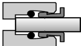
3. Push the tube firmly through the 'O' ring until it bottoms on the tube stop, then pull back.
