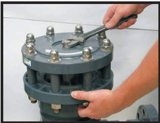
Backwash Flow Control Valve - rotate the adjustment bolt to increase or decrease flow/back-pressure
