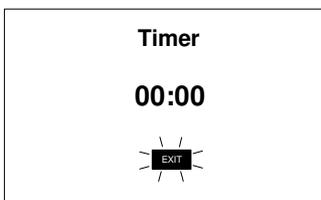
Key in the time required in minutes and seconds, maximum 29 minutes and 59 seconds, using the numerical keys, then select 'START' to start the timer. Use the **←** and **→** keys to reposition the cursor and re-enter the time if it is keyed in incorrectly.
