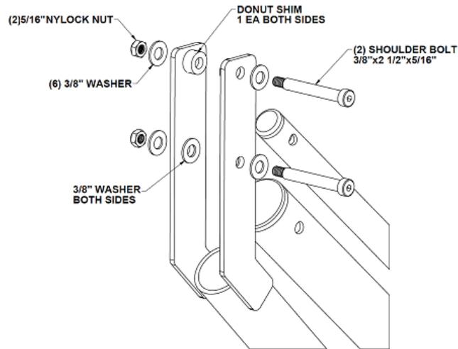
g. Attach the seat half and the seat belt to the mounting plate of the seat arm using:
