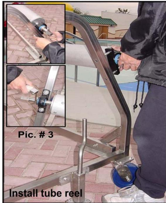
6. To prevent tube reel from moving laterally, slide shaft collar and set it firmly against the bearing and tighten set-screw on shaft collar. Repeat process on all other shaft collars. See inset on Picture #3.
