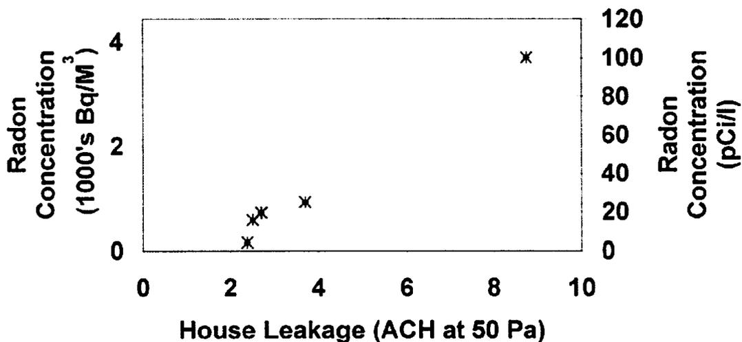
Figure 3: House air leakage versus winter radon concentration.
