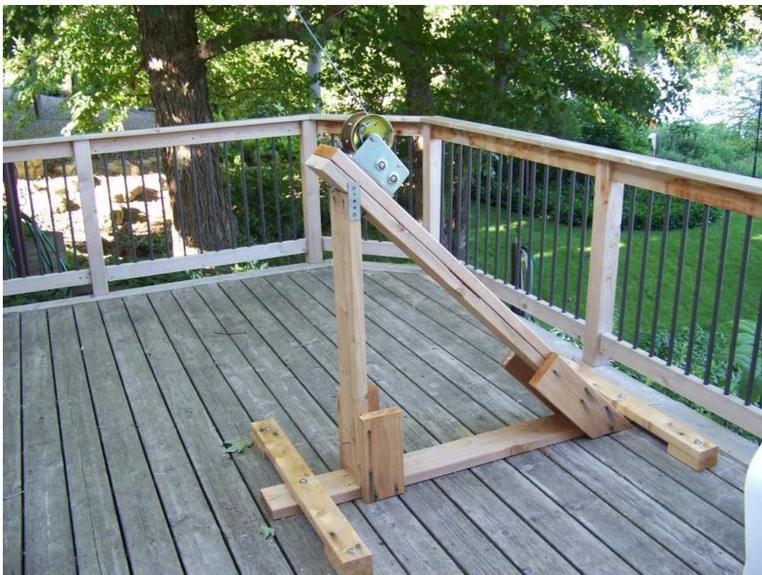
Falling derrick made from two sections of a telescoping TV mast that I have been saving for 35 years.
