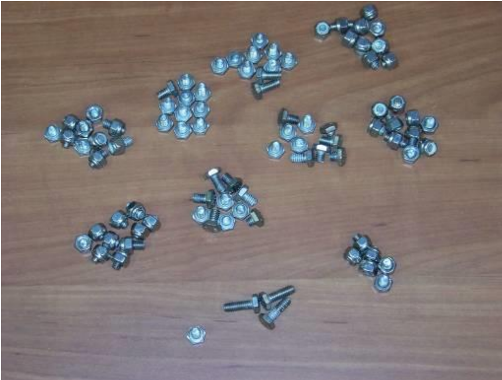
Collection of seized and subsequently broken bolts and nuts. A few bolts were recovered but unusable.
