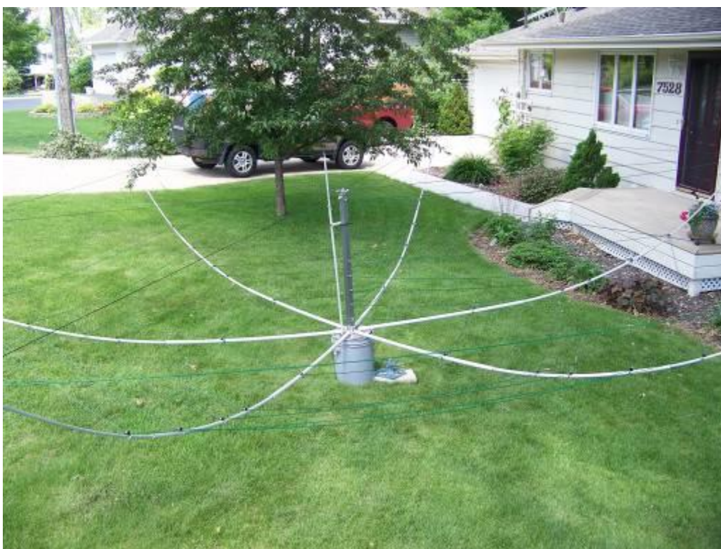
Assembled antenna, with the lightning rod attached.
