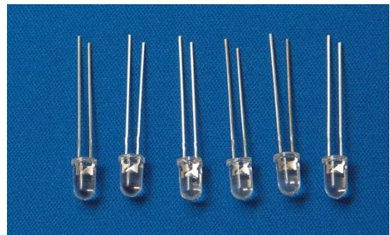
Figure 31 Six different colored LED's - long lead is +
