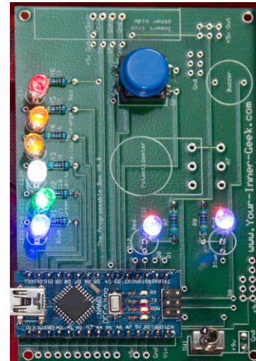
Figure 13 LED's all in correct locations - BUT NOT SOLDERED
