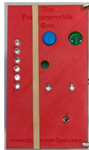
Figure 15 Hold top and PCB together with rubber band while soldering LED's
