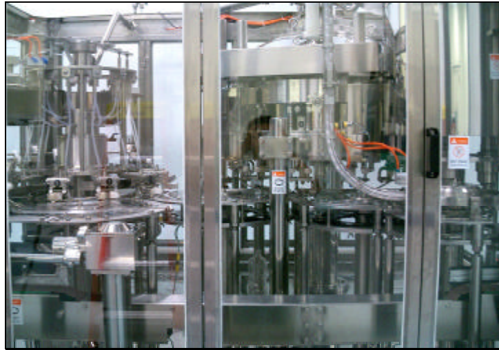
Rinser/Filler/Capper Close Up View
