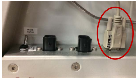
Figure 13 – Service bracket showing the RS-232 Communication port connection point.
