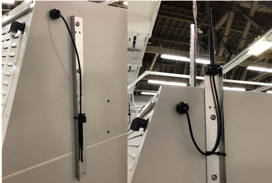
Figure 7 – Antenna shown in shipping position (left) and in operating position (right).
