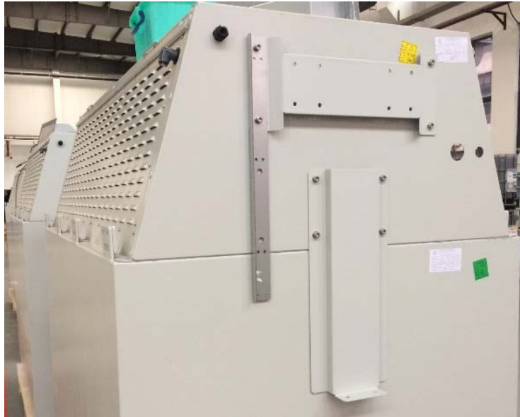
Figure 9 – PCS mounting bracket, installed.
