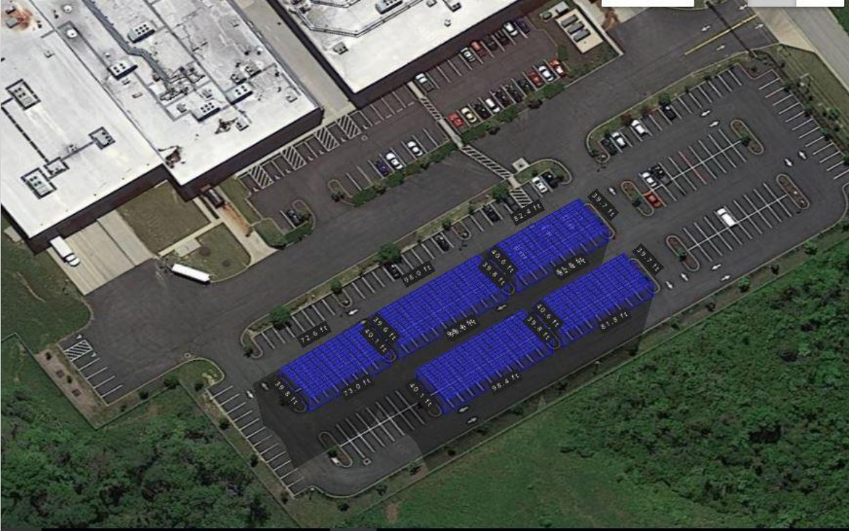
Closeup 3D view of a 260kw Solar Carport with REC290TP panels
