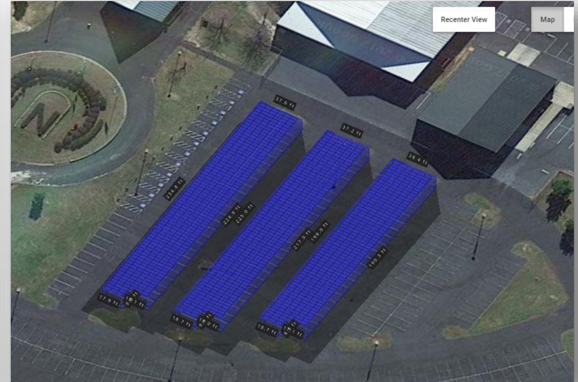
3D View of a 333kw Solar Carport
