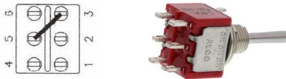
Now ensure that the Keyway is at the top as the drawing, then the numbering will be correct.
