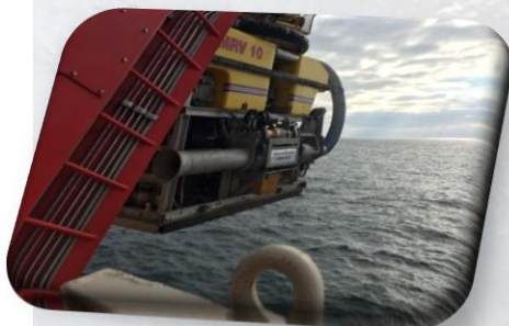
Picture Left shows a Predator MKI T6-8 Hybrid side mounted to Triton MRV ROV
