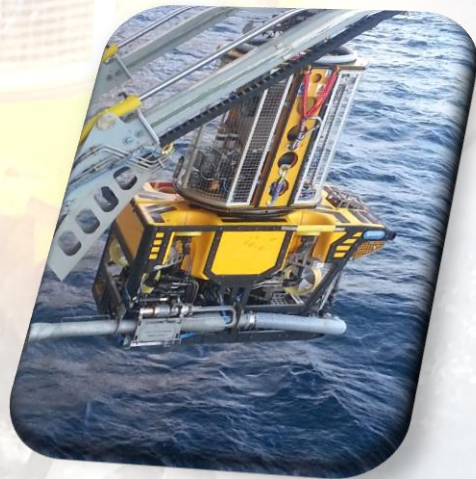
Picture to the right shows a Predator MKI T-8 mounted to SMD Quantum ROV
