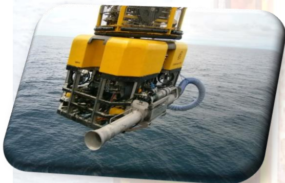
Picture to the left shows a Predator MKI T6-8 Hybrid dredger mounted to a Centurion HD ROV
